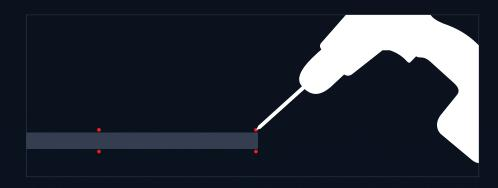
Using installation wire, beading wire, or fishing line, feed the wire from behind the housing/bezel, up and over the strip, then back down through the housing / bezel. Secure the strip by twisting the wire behind the housing or bezel.
