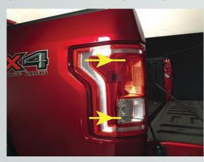
3. Disconnect the factory plugs from the factory tail light bulb sockets.
