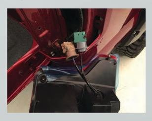
5. Secure the resistor box to the truck's sheet metal using the fitted 3M tape backing.
