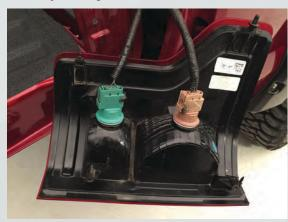
4. Connect the XB LED tail lamp plugs to the factory harness.
