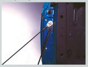
2. Remove the tail light by applying firm pressure to release the push-clips.
