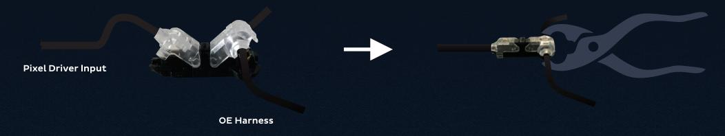
DRIVER ORIENTATION: The Pixel DRL driver must be plugged in so that the shorter output connects to the DRL board directly. The input and interrupt wires do not connect to the DRL board.
